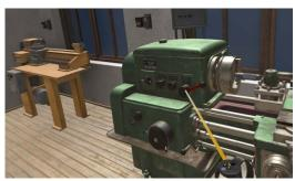
Carriage Auto Longitudinal turning can be moved in two directions i.e. forward and backward. For moving Carriage on Auto the user is required to point the controller to Mechanical Feed Joystick and it will be highlighted in red color then the User can move the Thumb-Stick on the controller to left towards Head-Stock or right towards Tail-Stock.
