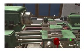
Chuck Speed can be controlled in four ranges i.e. Low Speed, Medium Speed, High Speed and Very High Speed. For selecting the Chuck Speed the user is required to point the controller to Spindle Speed Range Handle and it will be highlighted in red color then the User can move the Thumb-Stick on the controller to left or right side for selecting the four speed ranges.
