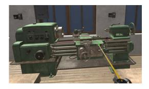
To rotate the Lathe Chuck point the Touch controller to the Spindle Rotation Control Handle and it will be highlighted in red color. Then the User can move the Thumb-Stick on the Touch controller Up for Clockwise, or Down for Anti-Clockwise rotation.
