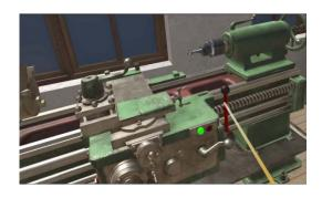
Carriage Auto Cross Slide can be moved in two directions i.e. Upward and Downward movement. For moving Carriage on Auto the user is required to point the controller to Mechanical Feed Joystick and it will be highlighted in red color then the User can move the Thumb-Stick on the controller to Upward or Downward for moving the carriage on auto.
