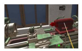
Carriage Longitudinal turning can be moved in two directions i.e. forward and backward direction. For moving Carriage the user is required to point the controller to Saddle Manual Travel Handwheel and it will be highlighted in red color then the User can move the Thumb-Stick on the controller to left or right side for moving the carriage.
